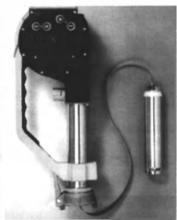
Measures ullage, innage, oil-water interface and temperature
