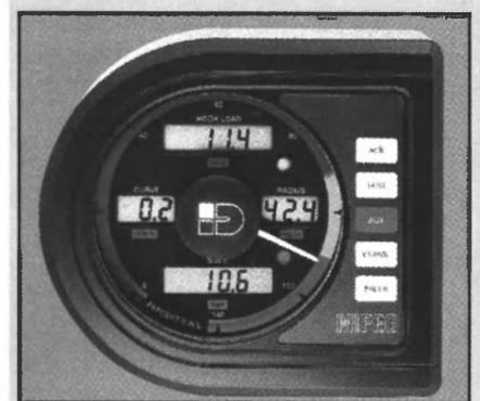
Datainstrument AS has introduced Mipeg 2000, an electronic load indicator and crane monitoring system designed to provide crane operators with the necessary information to meet worldwide government requirements for crane safety. The system comprises load, overturning and angle sensors with a micro computer that calculates the sensor data and provides an image of the crane's utilization on the operator's display.
