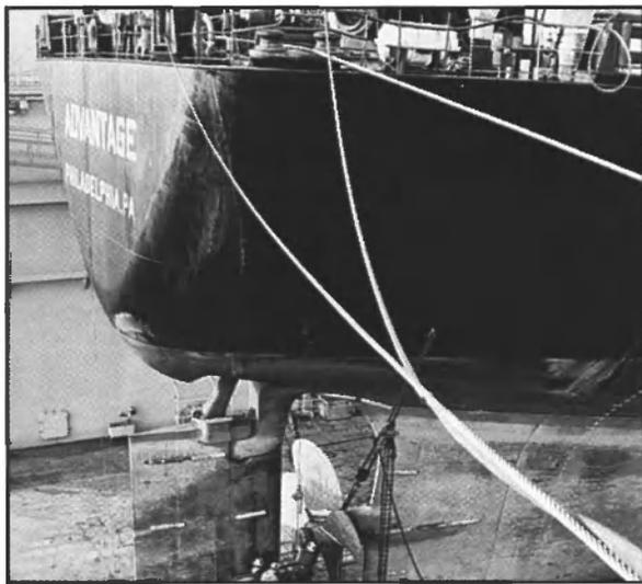
M/V Advantage, a 560-ft. (170-m) multi-purpose dry cargo ship, was recently equipped with a Thor-Lube stern bearing system.
