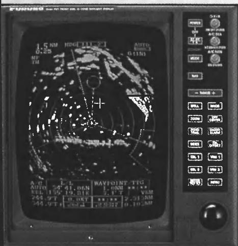
Furuno has replaced its FR7041 daylight viewing radar with an updated 12-in. X-band model the FR7061. The FR7061 reportedly provides a 50-percent increase in output power, a maximum range scale of 64 nm, optimized user-friendly software and True Echo Trail for accurate target tracking. Standard features on the FR7061 include dual EBLs and VRMs, EBL/VRM offset, off-center, zoom, echo trail, echo plot, and aural/visual guard zone alarm.
