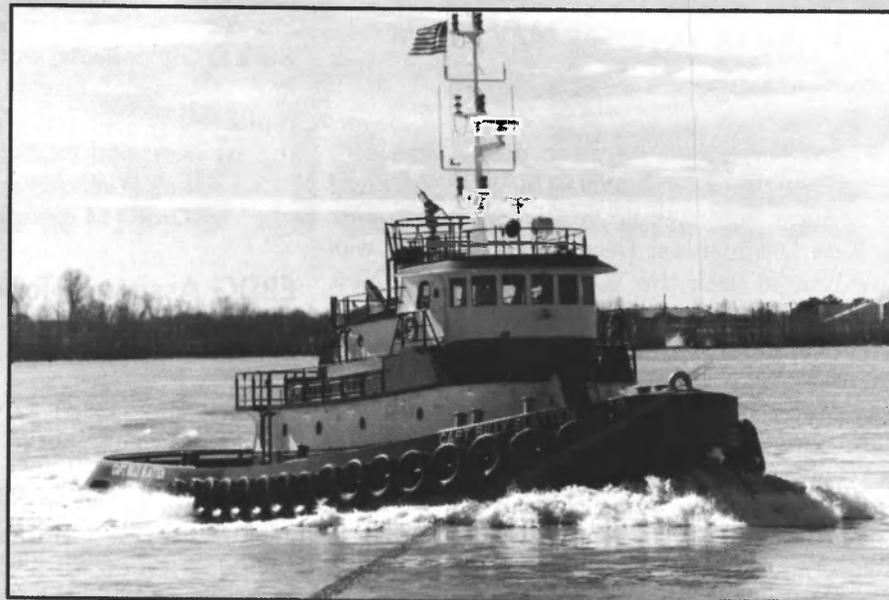
in tight spaces. This vessel is also outfitted with an stainless steel tow bits and bullnose, which will reportedly help prevent chafing and wear of the Spectra 900 fiber rope slings. This is the third tug in the Bisso fleet to be outfitted with these slings.
