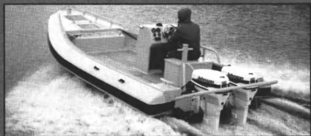
The external foam sponson is not only more durable, but also provides a large usable deck area, as shown on this AM 550 workboat.
