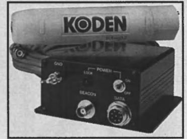
The Koden KBR-91 differential GPS beacon receiver is capable of pinpointing locations within 10 ft. by automatically locking onto the strongest differential beacon signal it can detect. The KBR-91 recognizes Type 1, Type 2 and Type 9 broadcasts, and it is compatible with the RTCM-104 interface on most differential-ready GPS receivers.
