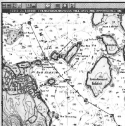
PinPoint Systems International has introduced Pinpoint Nautical Navigation, a charting system designed to utilize NOAA electronic charts on CD-ROM. PinPoint provides four communications ports for direct interface with GPS, Loran, autopilot, gyro, depth sounder or other navigational aids supporting standard NMEA data formats. All PinPoint systems include a NOAA prototype CD-ROM disk set that contains more than 150 official charts.
