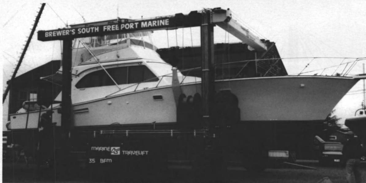
A Marine Travelift model 35BFM mobile boat hoist at work in Brewer's South Freeport Marine.
