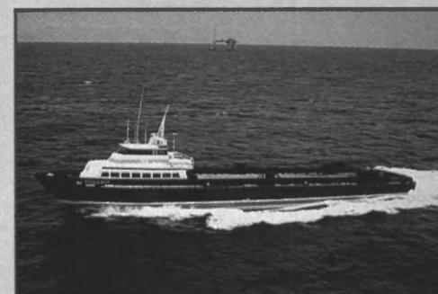
With a 30-ft. (9-m) beam, four V-12 KTA 38 Cummins engines easily fit across Paula Kay's engine room. Diamond Services put the 170-ft. (51.8-m), Hamilton jet-powered boat into service in Gulf of Mexico offshore oilfields in June.
