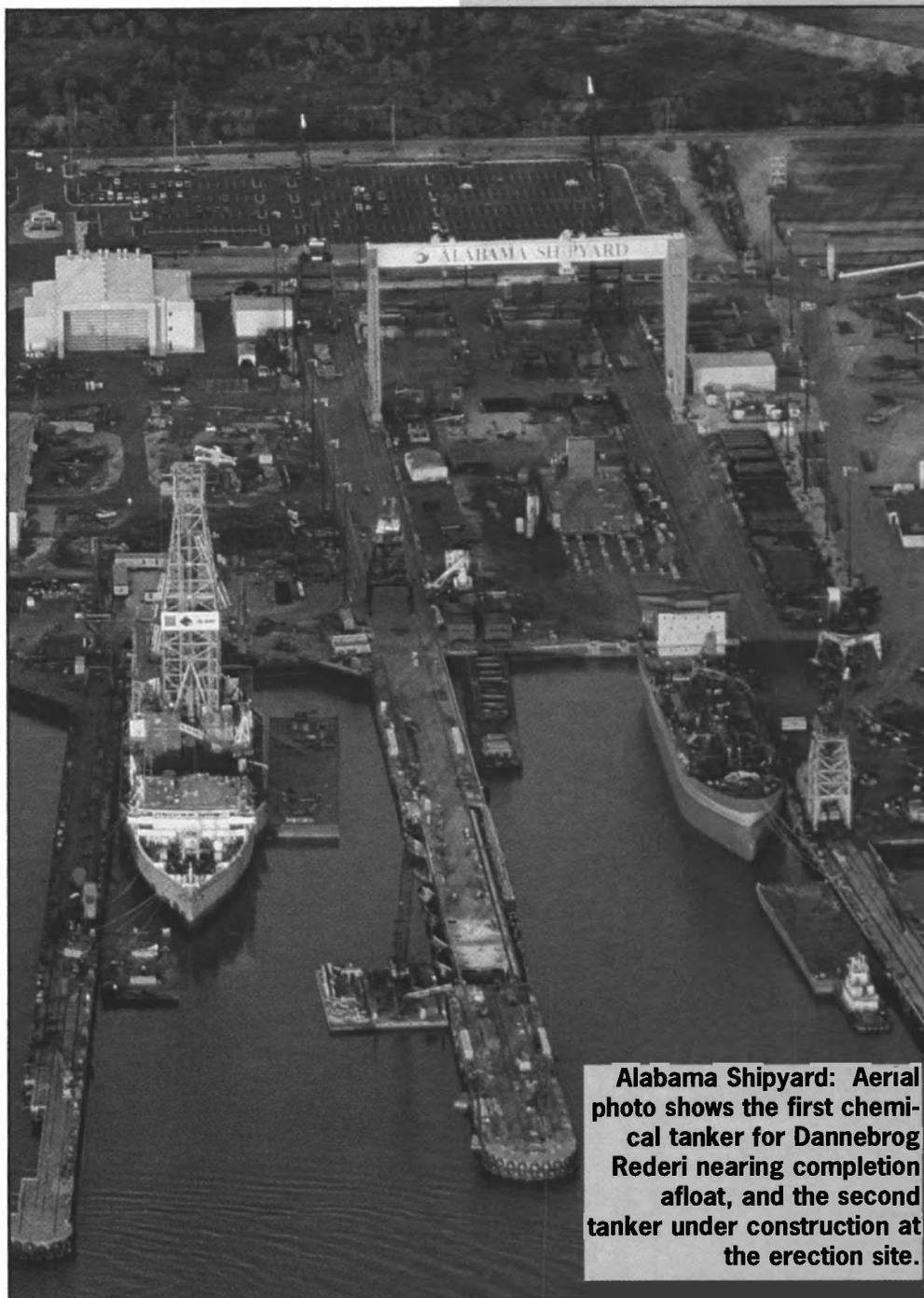
Alabama Shipyard: Aerial photo shows the first chemical tanker for Dannebrog Rederi nearing completion afloat, and the second tanker under construction at the erection site.
