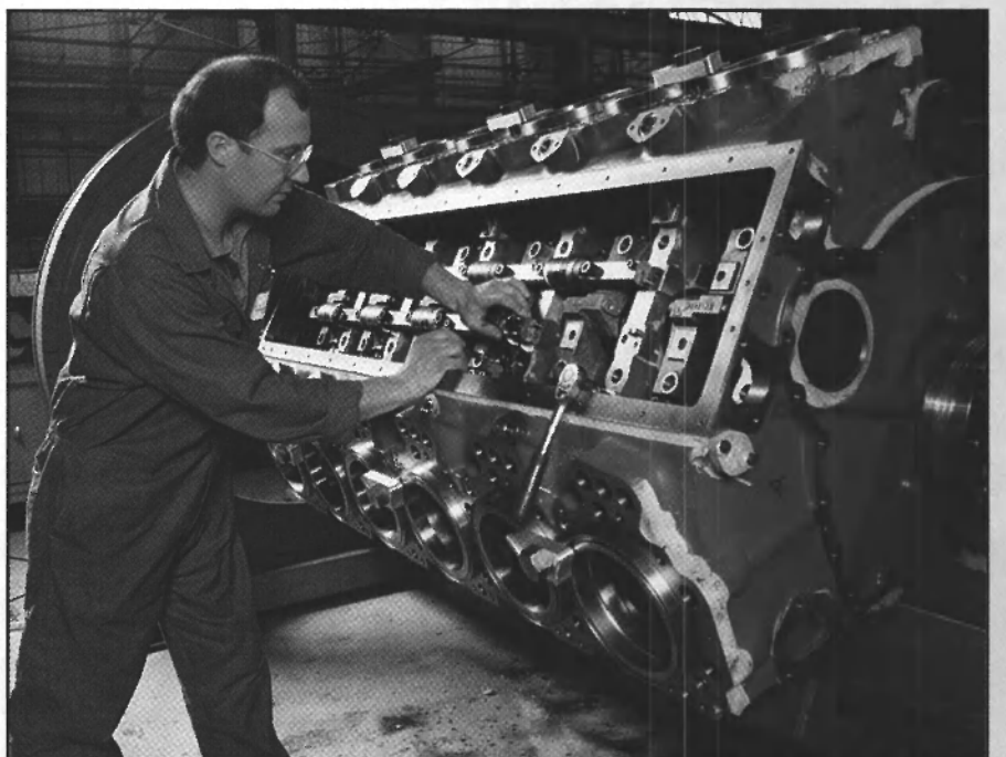
A Paxman 12VP185 high-speed engine is shown below, under assembly at the Colchester plant in the U.K.
