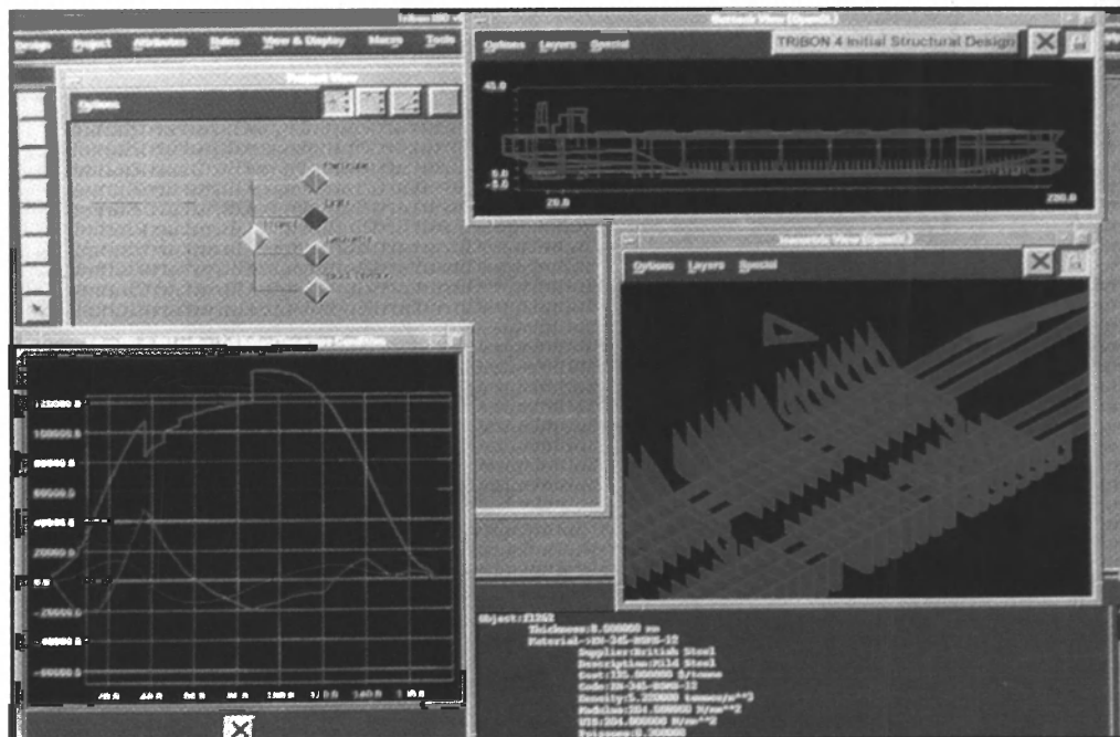
The Tribon Initial Structural Design. Lower left shows weight bending moment and shear force curves. Upper right shows preliminary structural configuration for a double bottom bulk carrier. The lower right shows attributes associated with a structural object.
