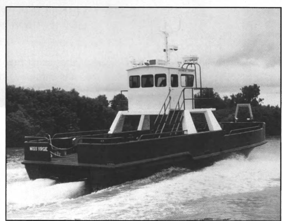
Miss Virgie features Twin Traktor Jet I-300 units.
