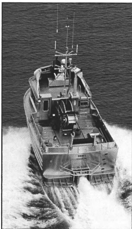
Erin L features the new Traktor Jet I-600HH.
