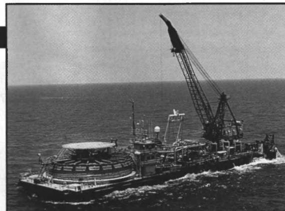
Global's reel pipelay barge *Chickasaw* laid both the *Arnold* and *Oyster* flow lines.
