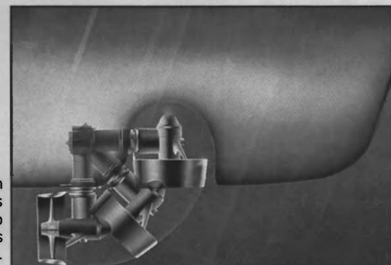
Right: The Ulstein Combi Thruster is swung down to operate in compass mode.
