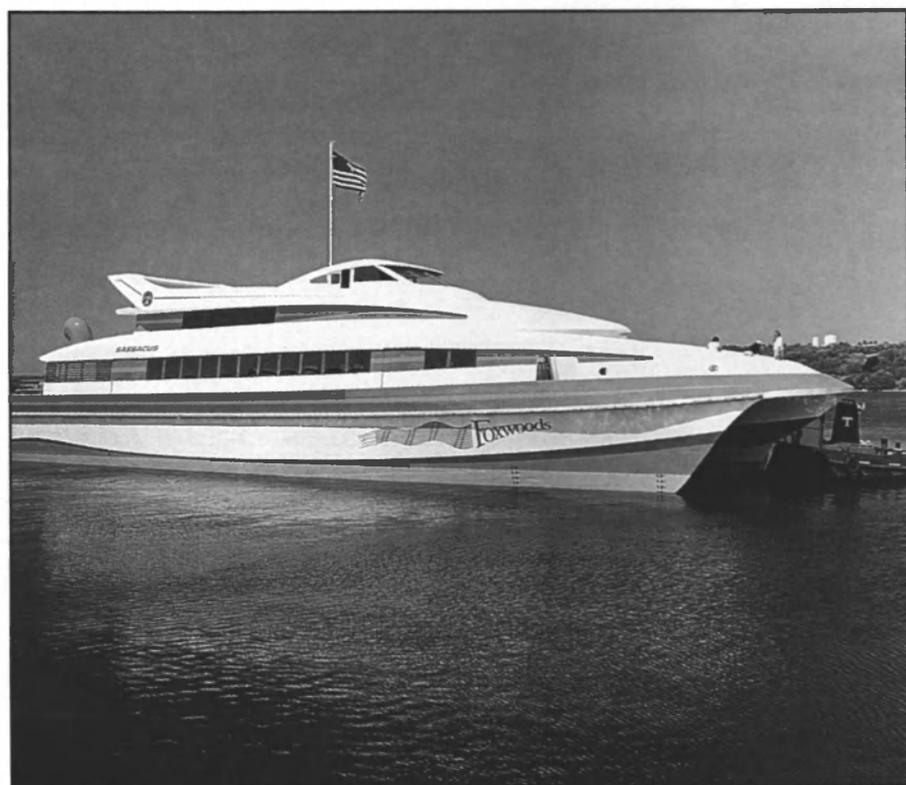
Hornblower Marine Services was scheduled to commence operations this month of what is touted to be the fastest passenger ferry in the U.S. *Sassacus* will make the 103 nautical mile trip from New London, Conn. to New York City in 2.5 hrs., traveling at speeds in excess of 50 mph. Built by Pequot River Shipworks, the new vessel complies with the new IMO High Speed Craft Code, as well as U.S.
