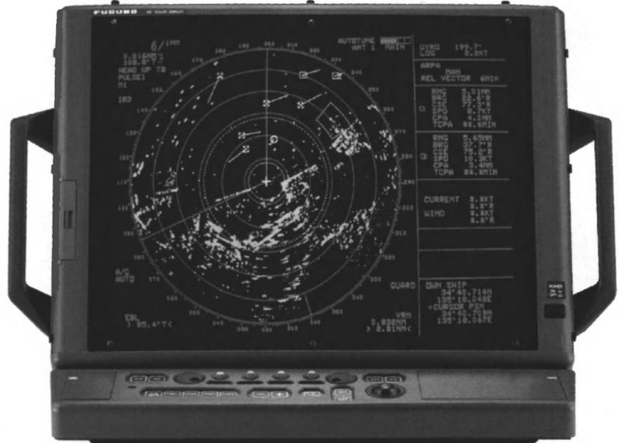
FAR2805 Series IMO-Compliant ARPA/Radar has both full-color and monochromatic displays
