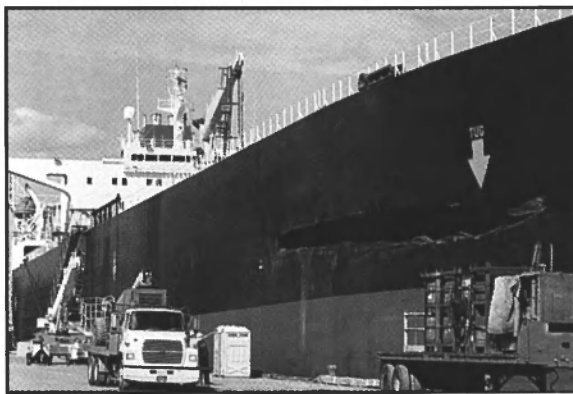
Pictured is Conoco tanker Guardian , featuring the gash sustained by the vessel during a recent collision.
