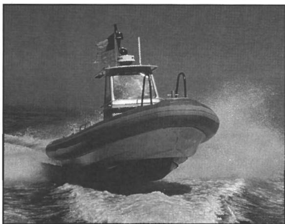
At the WorkBoat show held in New Orleans in November, SeaArk Marine introduced the new RAM class, soft-sided patrol boat featuring a D-shaped tube which can be filled with air or foam and allows for the use of the bow, side and quarter decks for boarding operations. Launched in a 24-ft. (7.3-m) model, the RAM class is available in various sizes up to 28-ft. (8.5-m) long.
