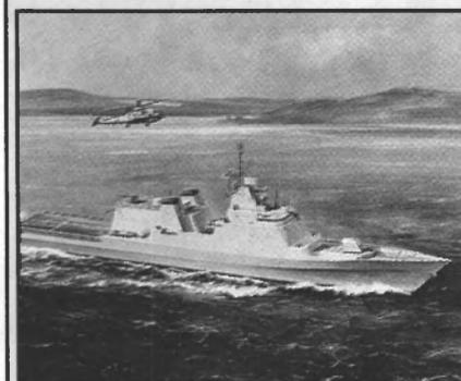
U.K. naval shipbuilder Vosper Thornycroft (VT) has designed an offshore patrol vessel (OPV) based on leading-edge technology developed for corvettes built for service with the Royal Navy of Oman in the Arabian Gulf. The design is the basis for the 285.4 ft. (87 m) patrol vessel required by the Royal Malaysian Navy (RMN) and the 272.3 ft. (83 m) OPV being sought by the Philippine Navy.
