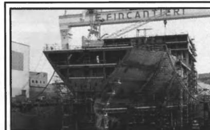
**FROM TWO TO ONE:** Disney's two cruise ships were each built in two sections at two different shipyards — Fincantieri's Ancona yard and Fincantieri's Marghera yard — in order to complete the vessels as quickly as possible.
