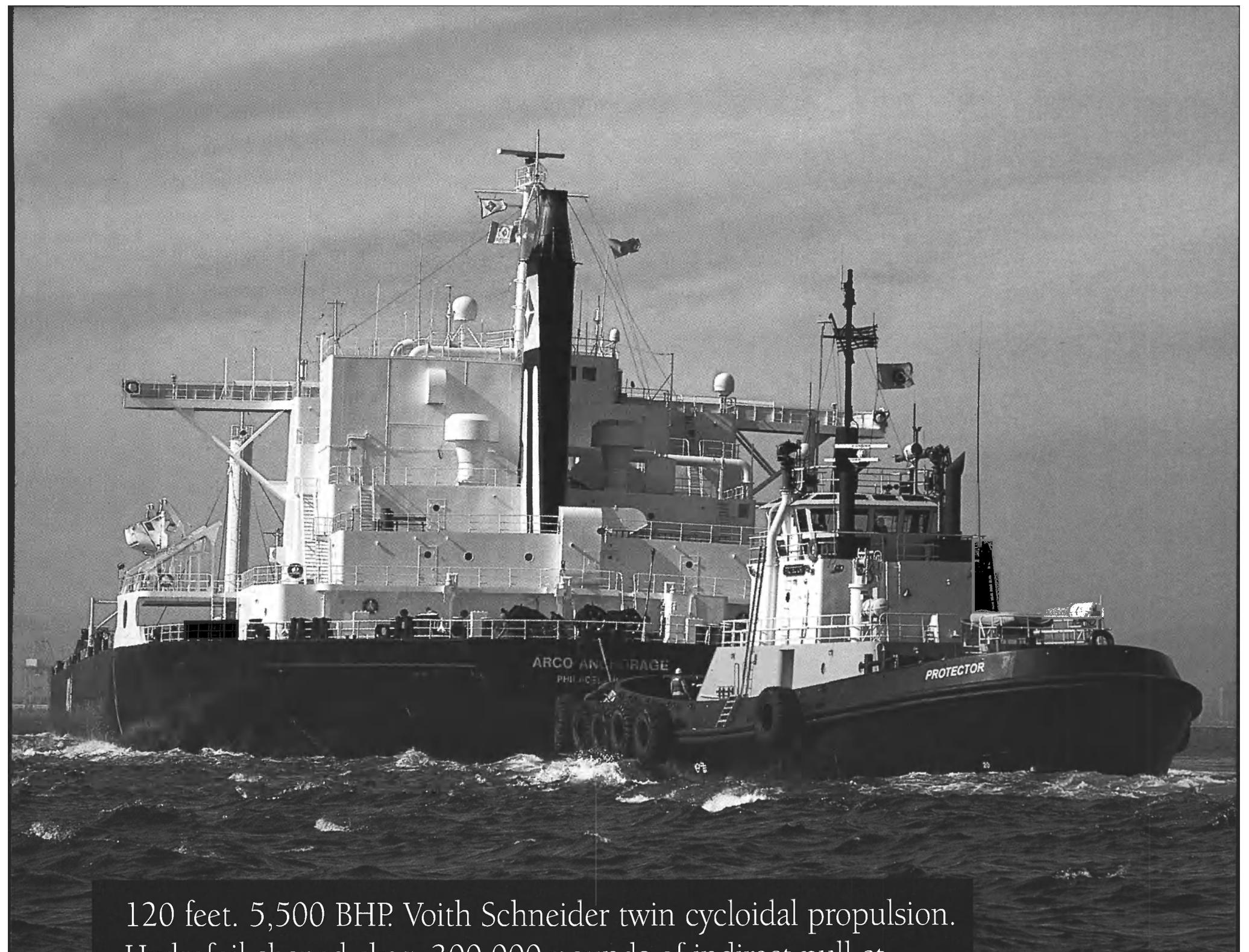
120 feet. 5,500 BHP. Voith Schneider twin cycloidal propulsion. Hydrofoil-shaped skeg. 300,000 pounds of indirect pull at 12 knots. More than just another answer – it's the solution.
