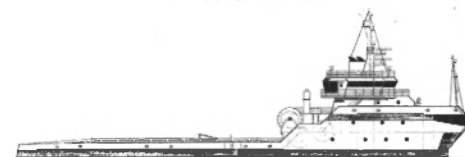
220'x48'x20' 8000 HP Anchor Handling Tug Supply Vessel
