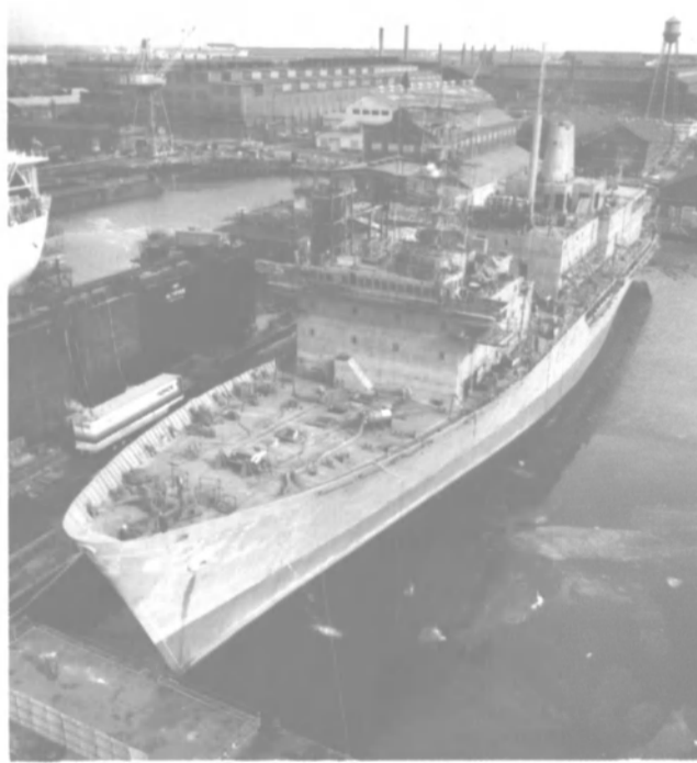
At left: Some of the 15 steel tunnel tube sections under construction at Bethlehem Steel's Baltimore Marine Division. The 300-foot-long sections will be used to build the Interstate 664 tunnel crossing in the Hampton Roads section of Virginia. At right: The USNS Maury (T-AGS-39), the first of two oceanographic survey ships being constructed at Bethlehem Steel-Sparrows Point. She is scheduled for delivery in July.
