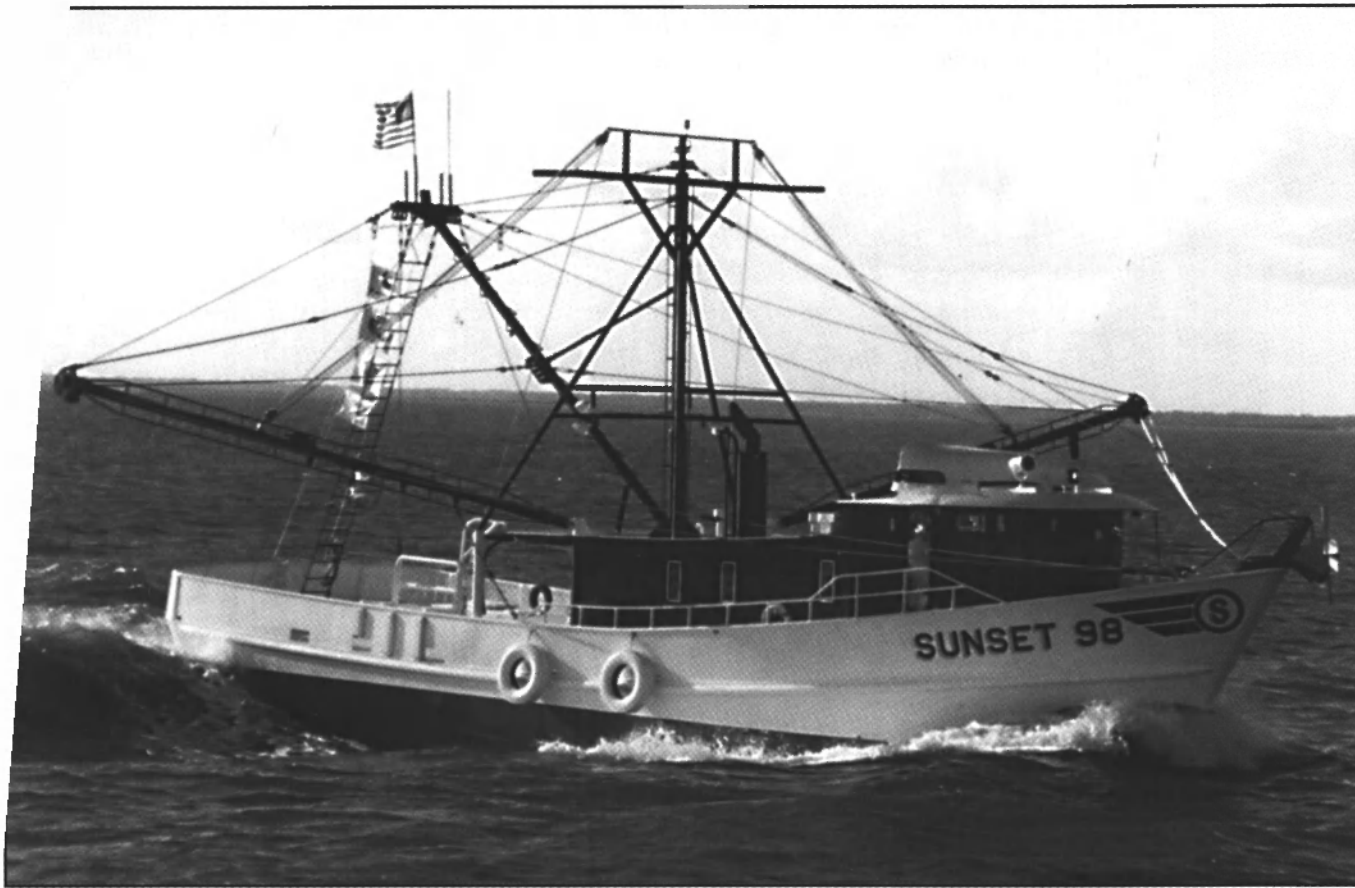
The Sunset 98 is the 160th 75' x 22' x 11' steel-hulled shrimp trawler built for the Sahlman fleet by Steiner Shipyard, Inc.
