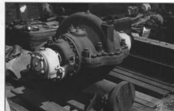
1 Cargo Pump Mfg: Ingersoll-Rand 3000GPM @ 150psi Horizontal Bronze Casing Model 8SHW Missing 500HP 1800RPM Motor
