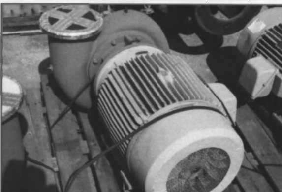
3 Circulating Pumps Size 8x8 Mfg: Carver 3000GPM@10.25psi Horizontal Bronze Casings Motor: Reliance 40HP 440/3'60
