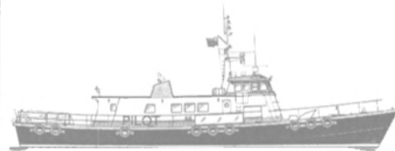
Outboard profile drawing of the new pilot station boats being designed and built by MARCO Shipyard Seattle.
