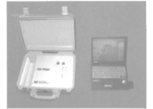
Saab Celsius TransponderTech's compact and portable AIS Pilot Case.
