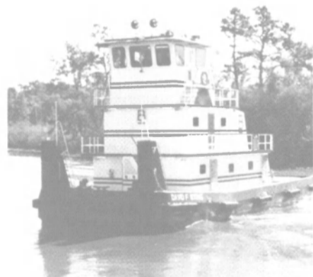
Measuring 65 x 24 ft. (19.8 x 7.3 m) David F. Stone, was constructed by Sneed Shipbuilding for Blessey Marine Services.
