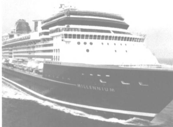
Measuring 965 ft. (294 m), Celebrity's Millennium is the first cruise vessel to house gas turbines.
