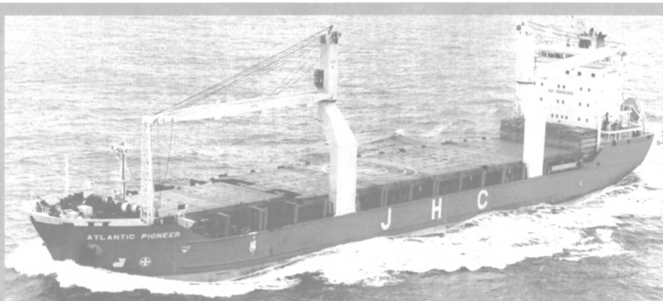
Atlantic Pioneer, the first in a 17,800-dwt series container-friendly multipurpose dry cargo ships built by a Chinese shipyard for Intership Navigation and feature MacGregor cranes.
