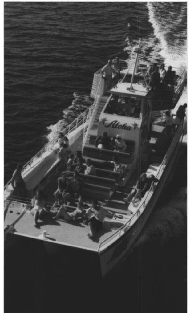
ft. (5.1 m), and is USCG approved for 71 passengers plus a crew of four. Powered by twin Cummins 6CTA diesel engines, driving 28-in. stainless steel propellers through ZF IRM 305A marine gears, Maui Magic will cruise at about 20 knots with a top speed of about 22 knots.
