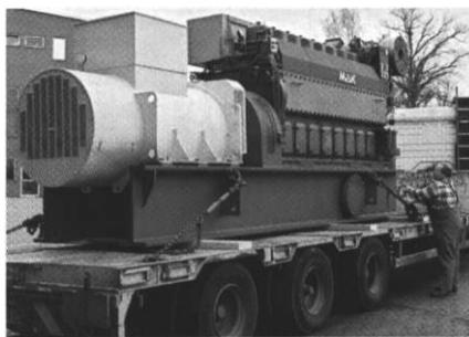
genset consists of Mak 8 M 20 with an output of 1,360 kW at 900 rpm for the container newbuilding 022 type WARNOW CV 2500. Since the acquisition by Kvaerner in October 1992, KWW has completed 35 container vessels, 32 of which were equipped with Mak diesel gensets of the engine series M 20 and M 25.
