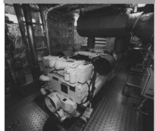
The vessel is powered by a pair of MTU 12V 2000M90 engines driving ZF gearboxes.
