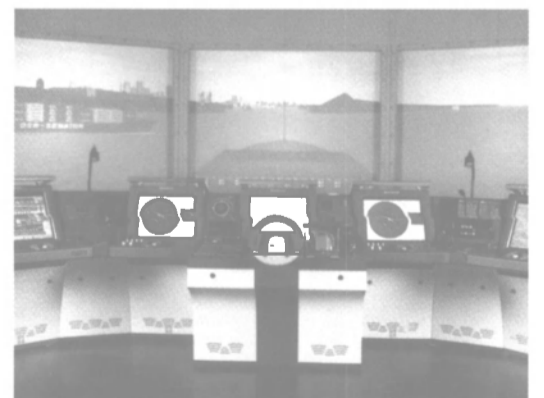
STN Atlas Marine Electronics' new Ship Control Center (SCC), developed for coastal shipping applications and incorporating NACOS navigation command system.
