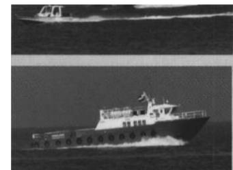
m) in length, with service speeds up to 30 knots. Robert Allan Ltd. provided Dubai Drydocks with a complete contract design package for the boat, based on the end-user's specific operating requirements. In addition, Robert Allan Ltd. provided with a complete set of production working drawings, including all parts and plate developments for NC cutting of all aluminium. Khulood was built to the approval of Lloyd's Register of Shipping.
