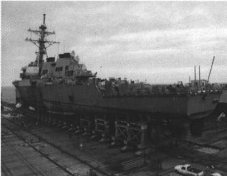
USS Cole was moved January 14 on land from Litton Ingalls Shipbuilding's floating drydock into a construction area of the shipyard's west bank.
