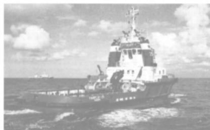
The latest Schottel tugs for the Fairplay shipping company are equipped with Schottel Rudderpropellers of type STT 1515 CP.
