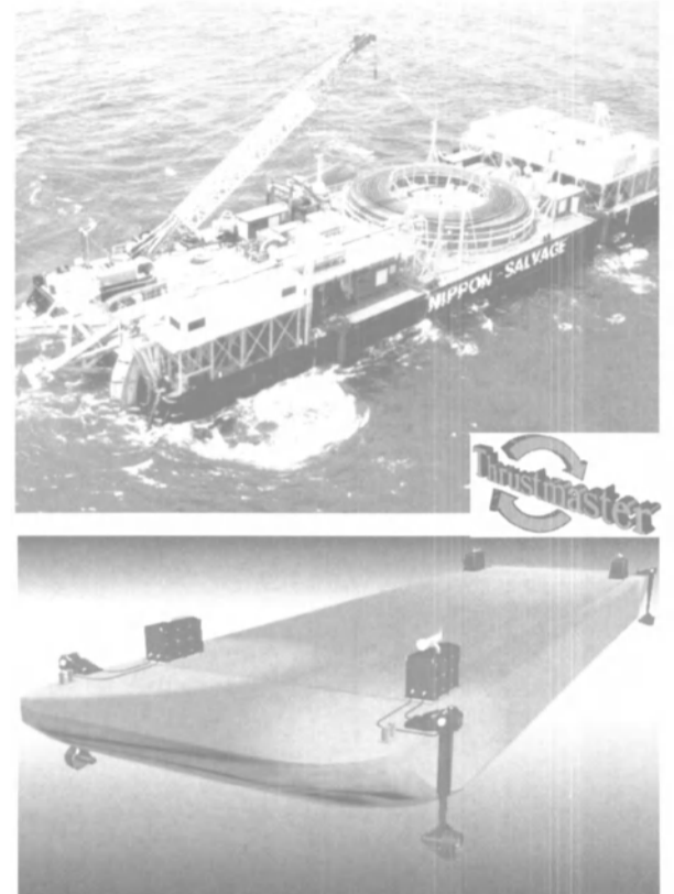
The PDPS solution from Thrustmaster offers cost effective solutions, as its use eliminates the need for dry-docking, structural changes to the vessel, and only takes a minimal amount of deck space.
