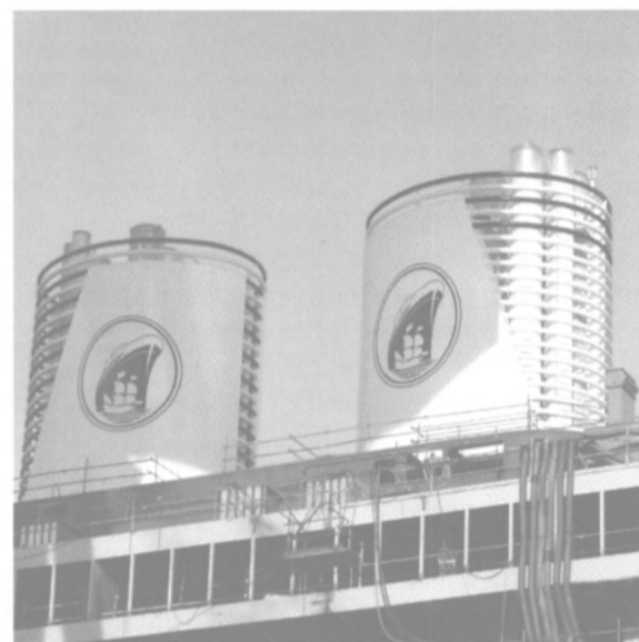
Constructed by Fincantieri, Holland America's Zuiderdam and Oosterdam vessels will boast two separate engine rooms with side-by-side funnels.
