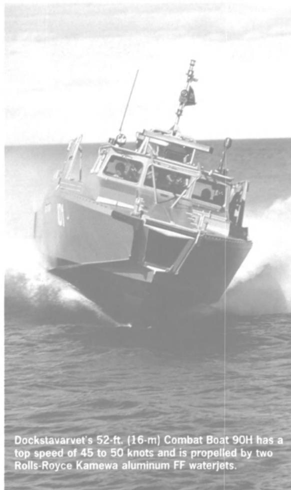
Dockstavarvet's 52-ft. (16-m) Combat Boat 90H has a top speed of 45 to 50 knots and is propelled by two Rolls-Royce Kamewa aluminum FF waterjets.
