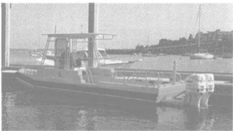
26/28 Center Console delivered to US Navy. Options include: removable top, soft sides & dive tank holders. Twin 150 Evinrudes w/48mph top speed.
