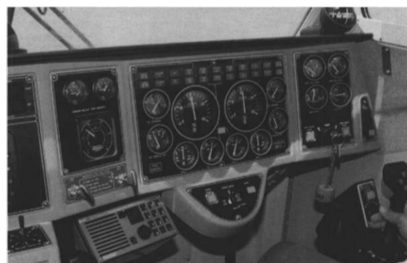
Typical instrumentation and controls in 3000TD, 4000TD and 8000TD hovercraft. Note the joystick control.
