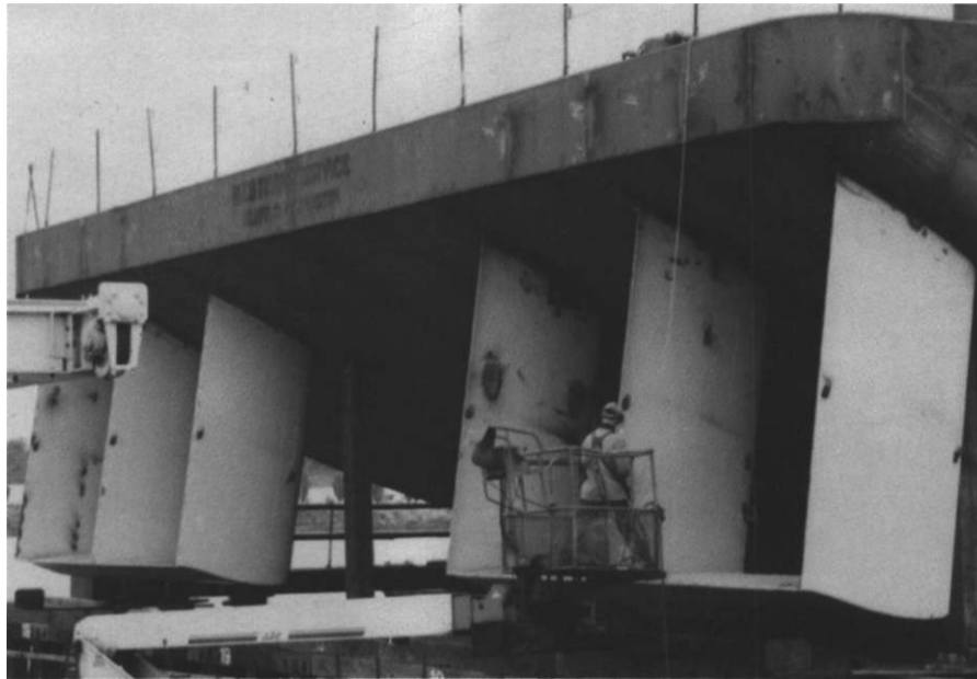
Invented by Joe Gruzling, President of Nautican Research more than 20 years ago, Hydralift skegs add 10 percent or less resistance.
