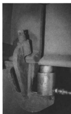
The Bulb-Align a tool for aligning Holland Bulb Profile Stiffeners when joining panel sections.
