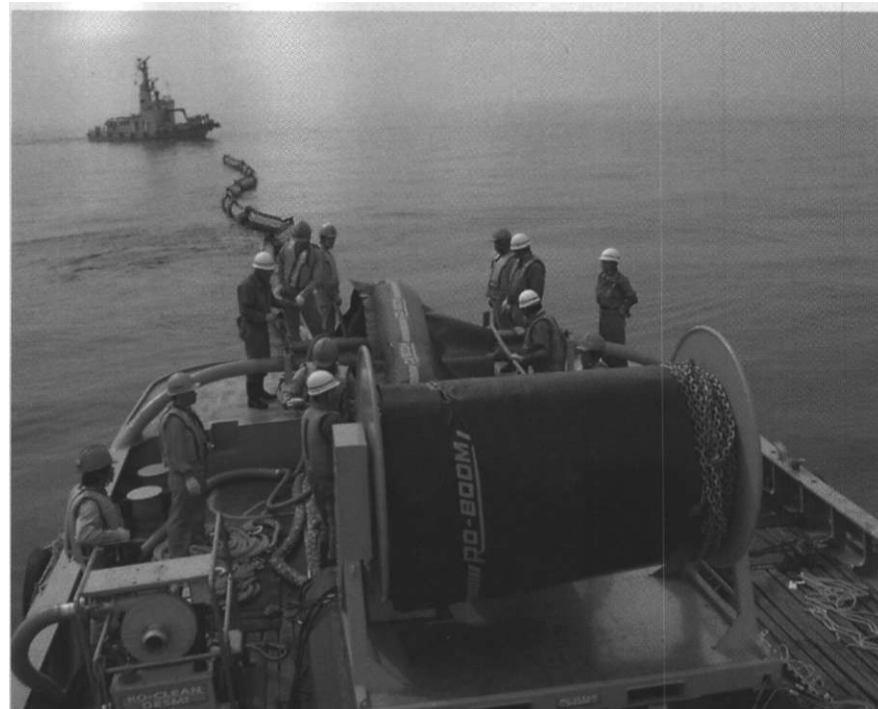
Oil spill response efforts for the Prestige sinking are being coordinated by Sasemar (Sociedad de Salvamento y Seguridad), which is a department of the DGMM (Dirección General de la Marina Mercante). Ro-Clean Desmi — a Danish manufacturer that has been making offshore booms and skimmers for over 25 years — has been on scene assisting, sending emergency teams with more than 16,700 ft. (5,100 m) of offshore oil containment boom during the first week.
