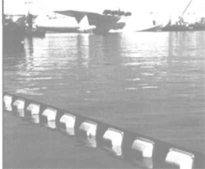
Port Security Barrier establishing a perimeter to control onlooking vessels during the transfer of Howard Hughes famous "Spruce Goose".
