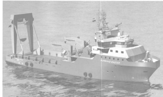
ers; two secondary winches with spooling device, and a 170-ton pull capacity; One storage winch for spar tow wire; twin stern rollers; two retractable anchor handling forks; and two sets of retractable towing pins.
