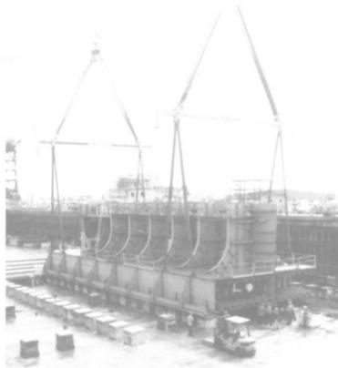
Double-hull configuration of Alaskan Frontier, which will feature twin-shaft diesel-electric propulsion.
