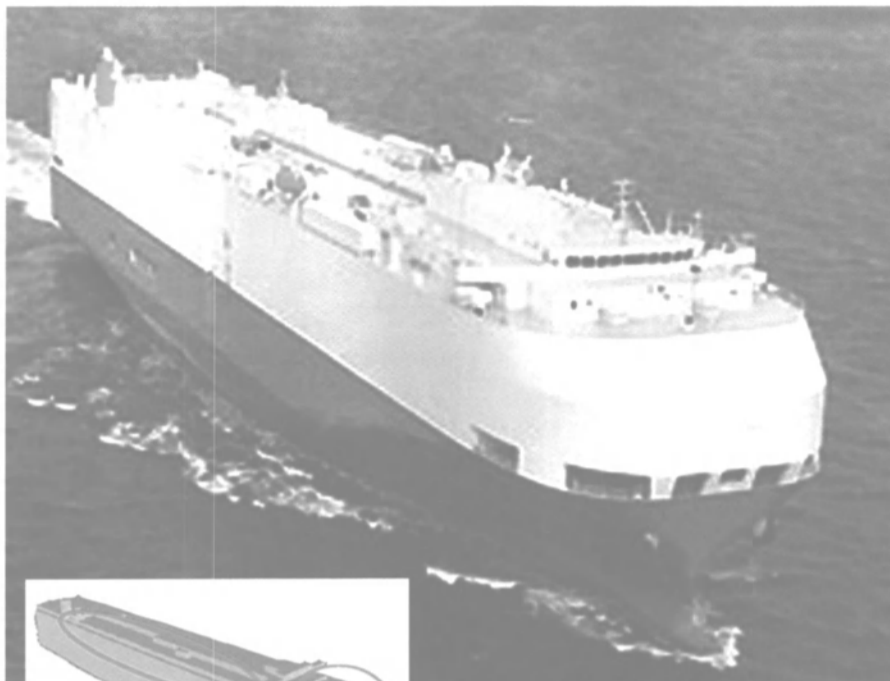
Above: The new 57,000-gt PCTC built for Mitsui OSK Lines by Minami Nippon Shipbuilding. Left: Image model of the PCTC, which depicts areas designed for less wind pressure resistance.
