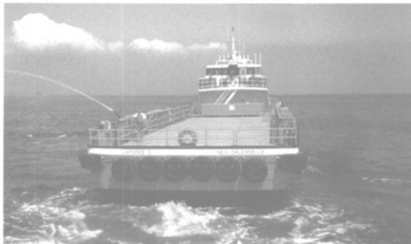
A. K. Suda, Inc. was approached by LaForce Shipyard of Bayou LaBatre, Ala. to design a crew/supply boat that would be faster, carry more deck load and more passengers and still be delivered at an economical price. The result is the 160 x 32-ft. (48.7 x 9.7-m) high-speed crew/supply boat that was recently delivered by LaForce at their Alabama yard.
