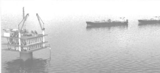
A patent-pending concept from American Shuttle Tankers dubbed Separate Storage Shuttling (S-S-S) envisions a unique shuttle tanker system for the Gulf of Mexico — serving a variety of floating production systems — that is cost competitive with pipelines.
