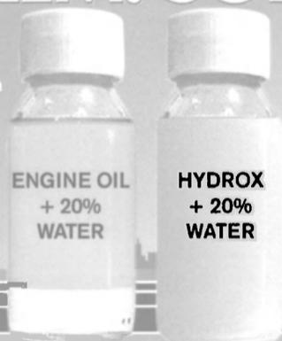
Hydrox forms stable emulsions which continue to provide effective lubrication even when significant quantities of water are present in the stern tube.
