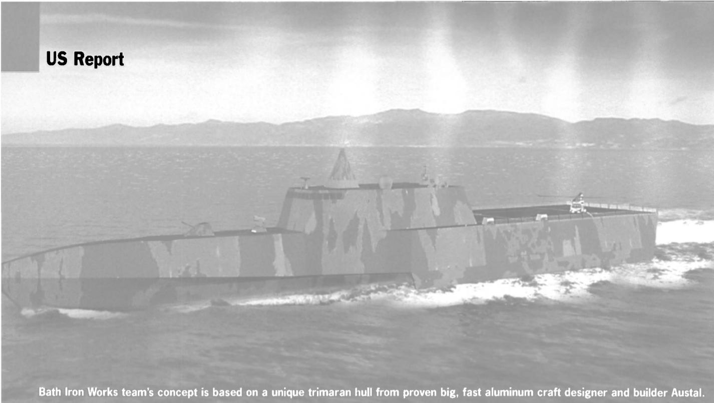
Bath Iron Works team's concept is based on a unique trimaran hull from proven big, fast aluminum craft designer and builder Austal.
