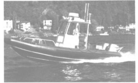
som dead rise and a 42-degree waterline entry point. The commercial models undergoing production are powered by twin 240-hp Yanmar diesels and Hamilton 274 waterjets.
