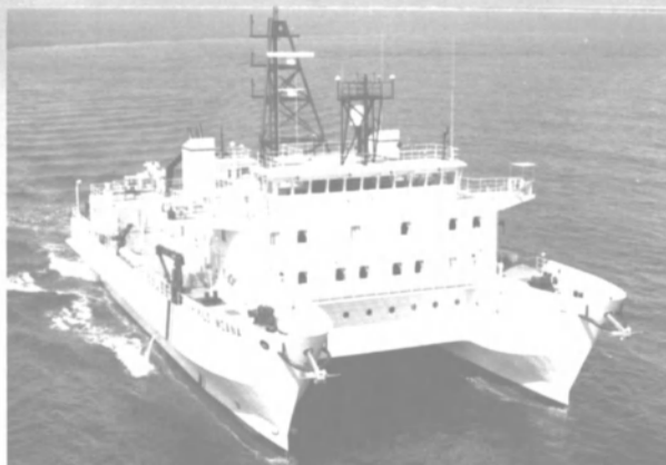
All-American - GPA recently (in partnership with Lockheed Martin), provided detailed design and engineering support for R/V Kilo Moana, a 185-ft. SWATH (small waterplane area, twin hull) oceanographic ship, which is owned by the Naval Sea Systems Command and operated by the University of Hawaii. Built by Atlantic Marine.
