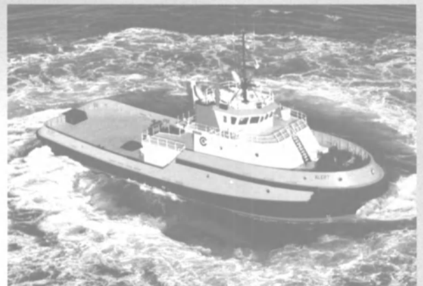
For Crowley Maritime's subsidiary, VMS, GPA provided preliminary, contract and detail design of the Alert, Attentive and Aware, all ABS classed and USCG inspected, for service in Alaska. Propulsion is provided by two Caterpillar 3612B diesel engines driving two Kamewa Aquamaster US 5001 Azimuth Z-drives.
