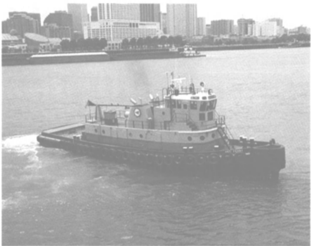
Crescent Towing's twin screw docking tug, Ned Ferry, on trials in the Mississippi River. It is the third of eight Crescent Towing 105-ft. sister ships to undergo the same upgrades and modifications at Bollinger Algiers LLC, the New Orleans based repair and conversion shipyard facility.
