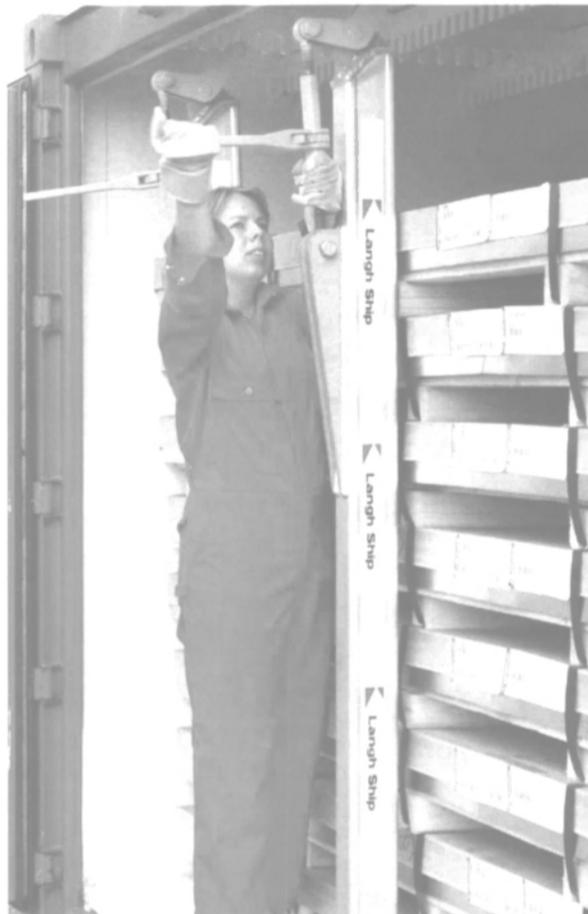
**Above** In Langh Ship's high container the load is secured with easily moveable stanchions fastened with a mechanism that has received a European patent.
