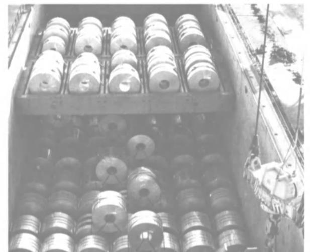
**Bottom Right** Pictured are heavy steel coils both in the traditional location at the bottom of the hold and higher up on the European patented cradle tween-decks.
