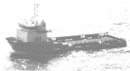
Seacor Madison, the first of three 207-ft., 4,750 bhp supply boats, was delivered to Seacor Marine, Inc., from Bollinger Shipyards, Inc. The boats are part of Bollinger's new 220 Class OSVs, vessels designed to raise versatility and cargo carrying capacity, while lowering operating costs.
