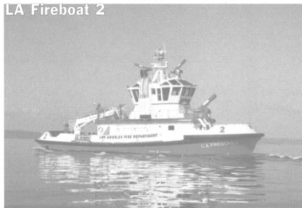
Propulsion and steering control are provided by twin Voith cycloidal propellers, Model 26 GII/165, provided by Voith Schiffstechnik, each driven by an MTU/Detroit Diesel Model 12V4000 diesel engine, rated 1,800 bhp (1,343 kW) at 1,800 rpm, which also drive a fire pump through a front end PTO. In addition, a pair of MTU/Detroit Diesel 8V-4000 pump engines each drives two fire pumps. All machinery is resiliently mounted for minimization of noise and vibration transmission.
