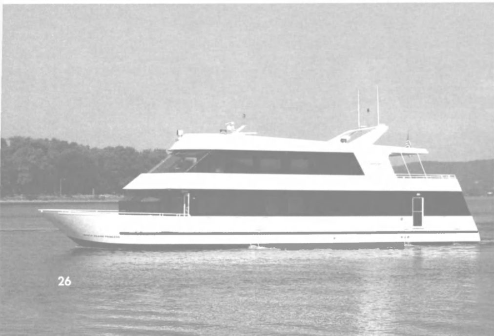
BELOW: One of several luxury charter yachts built by Skipperliner in 2003. This 80-ft. vessel is designed for smaller markets and can hold 149 passengers for excursion and cocktail service and 65 for seated meal functions. (Photo By Skipperliner)
