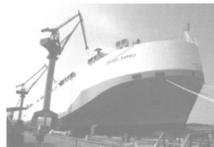
decks, its height is comparable to a 33-m building consisting of 11 floors. The engine power is 11,060 kW delivering a 20-knot maximum speed and a 19.3-knot duty speed.
