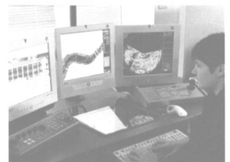
The Waterside Sentry System, developed by CompuDyne's Quanta Systems division, is an "invisible fence" comprised of radar, sonar and cameras. The Waterside Sentry System uses radar and sonar technology to detect a terrorist threat from the sea and instantly alerts
