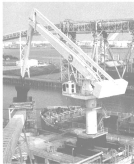
The E-Crane® (Equilibrium Crane) is changing the basic concept of how ships are unloaded in ports around the world. It is an advance that has proven it moves more bulk material faster, farther and at lower cost than any conventional crane type.
