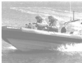
Ribcraft's Mitigator 25 ft. (7.8 m) vessel is a popular choice for the U.S. government, selected by the U.S. Coast Guard and U.S. Air Force recently. The new 25 ft. Ribcraft Mitigator integrates multiple technologies designed to enhance driver and passenger comfort and safety by mitigating many of the naturally occurring actions generated by changing sea conditions and high speeds.
