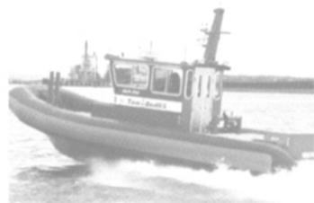
The quick response rescue RIB, Safe/Sea Block Island, measures 33 x 12 ft. and was built by Almar for Safe/Sea. The Almar hull is welded marine aluminum of heavy duty construction, and features 28-in. diameter Wing polyurethane tubes; twin 315 hp Yanmar Diesel engines; Borg Warner 1:1 gears; and Hamilton 274 jet propulsion units.
