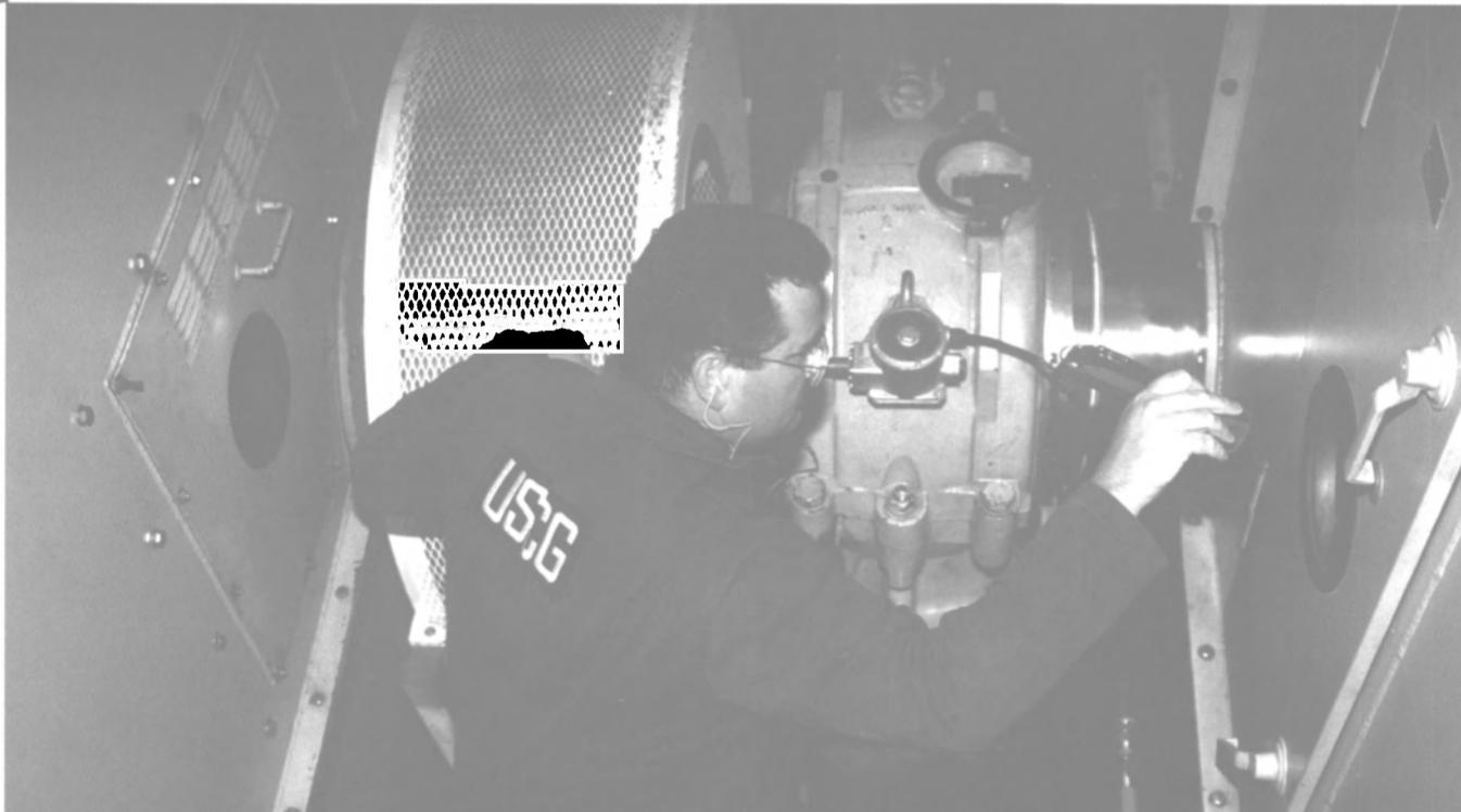
ago, in an attempt to lessen the amount of waste oil entering the ocean from ships, the international community required most ships to install and operate oily-water separators (OWS). An OWS separates oil from the rest of the liquids by means of gravity, centrifugal force, osmosis, or other process or combination of processes. Originally, the devices were designed to operate at 100 parts per million (ppm). Now, they are
