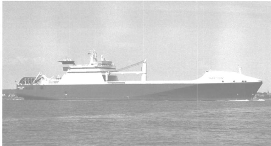
Flensburger has significant experience in delivering advanced combined carriers, as evidenced by its RoRo 2700, a 13,300-dwt, 22-knot, 2,700 lane meter ship.
