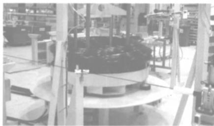
Many of T-DRILL's tube cut-off machine customers are considering the use of the large diameter coils. By pulling the tube from the center of the coil through the so called "eye in the sky" handling system, the tube can be fed from the coil and allowed to naturally orient prior to entering the system straightener.
