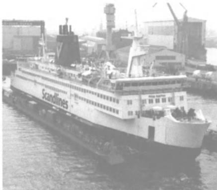
On August 17 the 152 x 23.12 x 5.64 m Danish Baltic Sea ferry Prins Joachim was floated into Dock 16 of Blohm + Voss Repair GmbH. In the course of the docking period, the ferry of Scandlines Denmark will be equipped with more powerful engines — six MAK main engines with a total power of 23,000 kW — allowing the ferry to reduce its crossing time on the Rostock to Gedser (DK) from 120 to 105 minutes.
