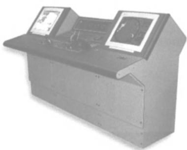
(Voice on LAN) - Intercom, VHF, MF/HF, UHF, Inmarsat B and Inmarsat C: VHF - Military VHF channels 39, 90 are implemented in the VHF station: Loran-C - New Man Over Board (MOB), signal strength and circular error probability functions.
