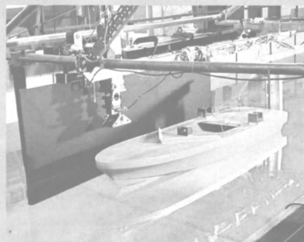
Test set-up for simulating Puget Sound Pilot Boat along side a ship. The sheet of plywood (with bootstripe) simulates the side of the ship. (Courtesy Vizon Scitec with permission)
