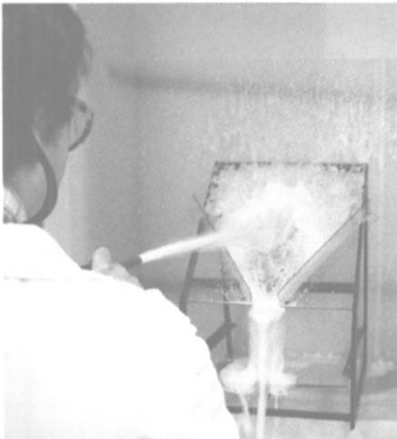
Drew Marine introduced a new program to analyze firefighting foam in fixed extinguishing systems, an extension of its marine products and services to help keep marine operators in compliance with international regulations that require firefighting foam to be periodically analyzed and certified.
