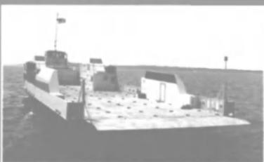
Hull 315: Isleño, 35' 3200hp, 14-18 knots, quad-screw shallow draft (7'-6" max), 400 LT capacity, 200 passengers, 4 trailers or 40 cars, ocean-route OSV-type vessel. Delivery: August 2004
