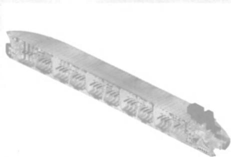
Section down the centre line of an NE Nastran full vessel model of a tanker, showing stress contours
