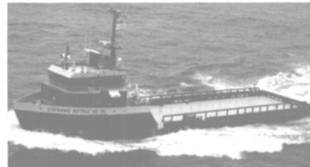
Cheramie Botruc 38, Bollinger Shipyards latest new 191-ft. platform supply boat that meets all new regulatory requirements including DPSI and is under 200 gross tons.
