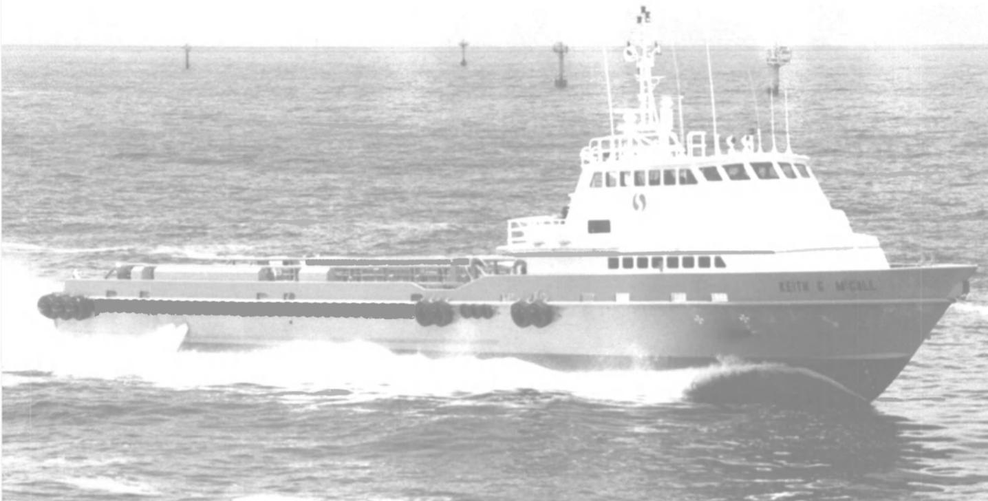
Neuville builds for Seacor. Main power is four KT-38 engines from Cummins each rated at 1350 hp that drives the vessel to 26 knots light speed. Twin Disc transmissions couple this power to four bladed Nibral 42-in. diameter by 48-in. pitch props. Light speed is 26 knots. Fuel capacity is 20,986 gallons and rig water capacity is 37,674 gallons. Passenger capacity is 81 persons in declivable seats.
