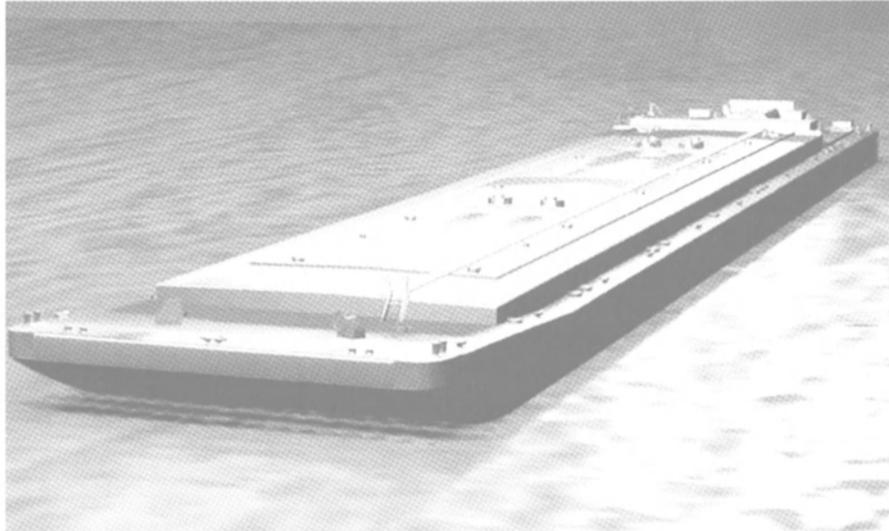
Artist drawing of the raked design 297.5-ft., 30,000-barrel (BBL), double hull, hot asphalt tank barges Bollinger is building for Horizon.
