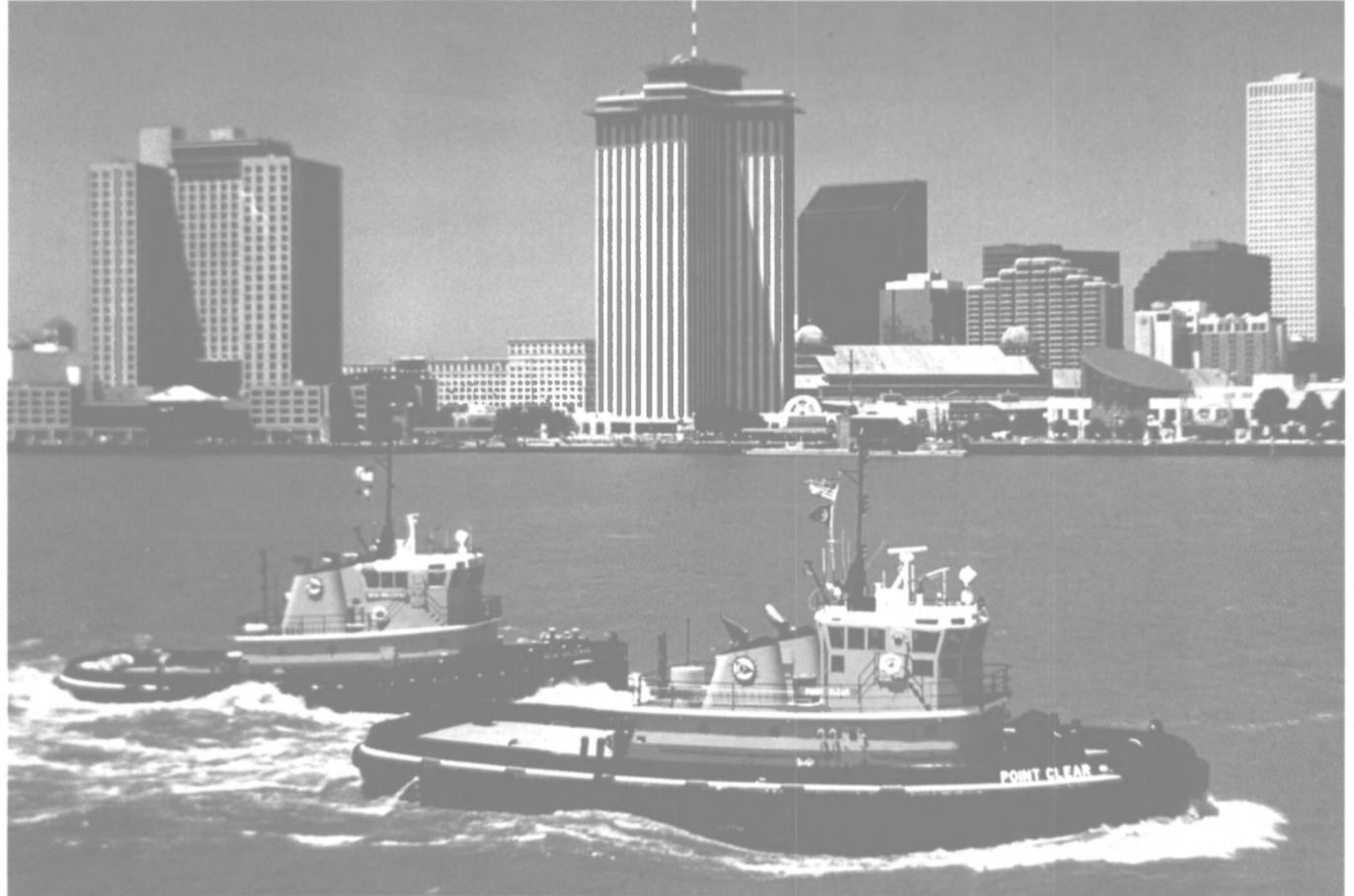
2,500 shaft horsepower (shp) each, and according to Ohler is the most powerful tug in New Orleans. The vessel has tankage for 85,000 gallons of diesel fuel, making it capable of prolonged towing assignments.
