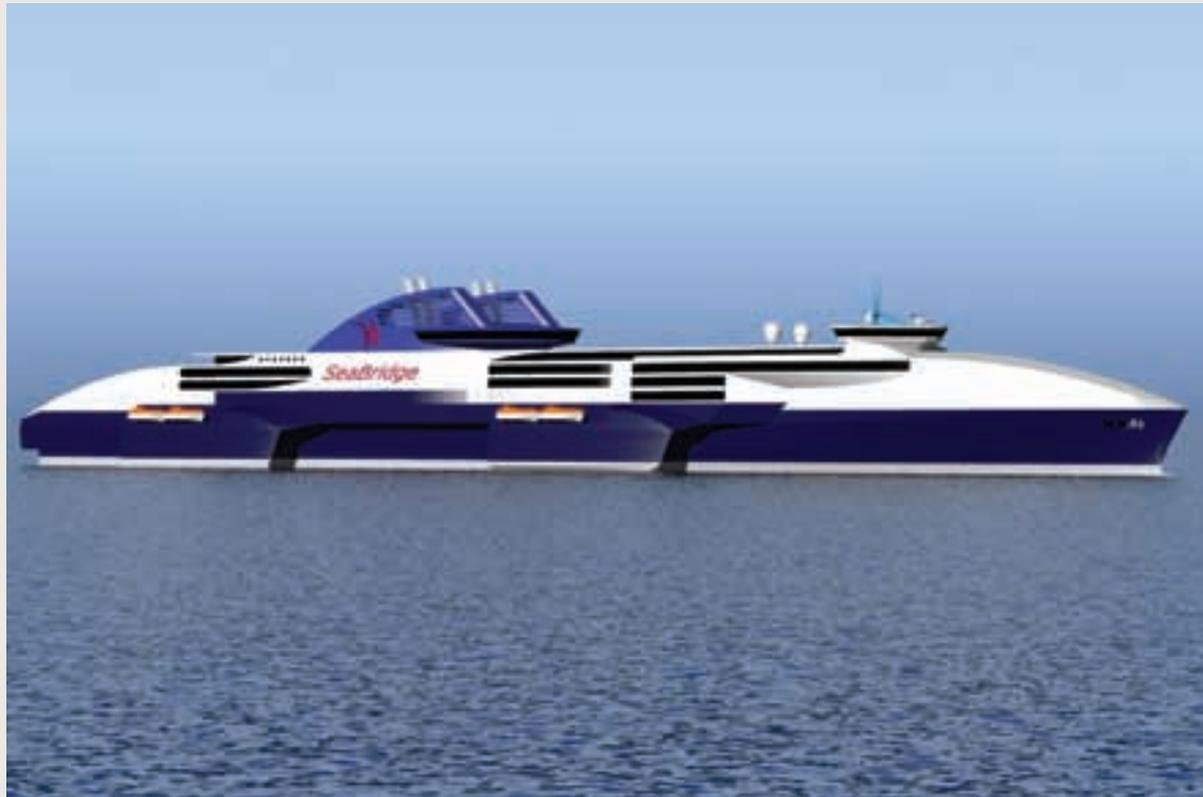
delivering electrical energy to five 31.5-MW propulsion motors driving five Lips waterjets. The layout is intended to ensure a 40-knot laden speed at 90-percent maximum continuous output of the main engines. Four of the waterjets would be steerable.
