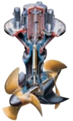
Drawing of a Schottel Combi Drive (twin propeller version)
