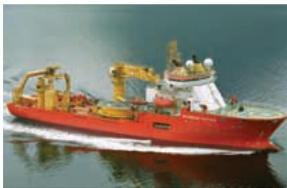
The cable laying vessel "Normand Clipper" will undergo an extensive conversion equal to that of its sister vessel "Normand Cutter". Here is the converted "Normand Cutter" immediately after its conversion was completed in May last year. (Photo: **Harald M. Valderhaug**). The conversion (below) started at Ulstein Verft in December 2004.
