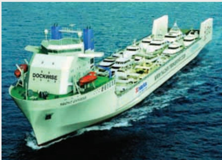
The new yacht carrier will be equipped with a 19,680 kW diesel-electric plant for propulsion, ancillary electrical power, and all shipboard electrical services. The plant will be powered by two Wärtsilä 12V38B main diesel generating sets, two Wärtsilä 6L20 auxiliary generating sets, and a 300 kW emergency generator set.
