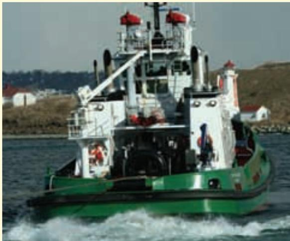
Two remote-controlled FiFi monitors supplied by FFS capable of a discharge rate of 1,200 m<sup>3</sup>/h each are fitted just aft and above the wheelhouse. The monitors are supplied by a dedicated pump of 2,700 m<sup>3</sup>/h capacity, driven off the front end of the port main engine. A water curtain of 300m<sup>3</sup>/hr is also supplied by the pump, or alternatively foam can also be supplied at 300 cu. m./hr.
