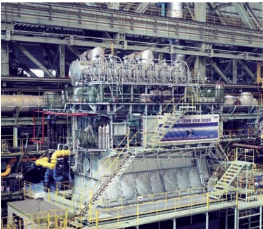
MAN B&W Diesel 7S65ME-C on testbed at Hitachi-Zosan after type test.
