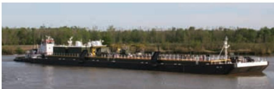
**DBL 28, the first in a series of eight OPA'90 compliant, Lakes, Bays & Sounds, ABS and USCG certified tank barges delivered from Bollinger to K-Sea Transportation for use in harbor service in ports on the Northeast U. S. Coast.**
