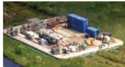
for use in Suriname in North Eastern South America where it is needed to facilitate oil exploration. The Hoverbarge is also able to carry 350 tons of exploration equipment at a speed of five knots over a variety of surfaces. The Hoverbarge is basically a large platform measuring 197 x 98 ft. (60 x 30 m) constructed of 21 steel boxes measuring 59 x 9.8 ft. (18 x 3 m).
