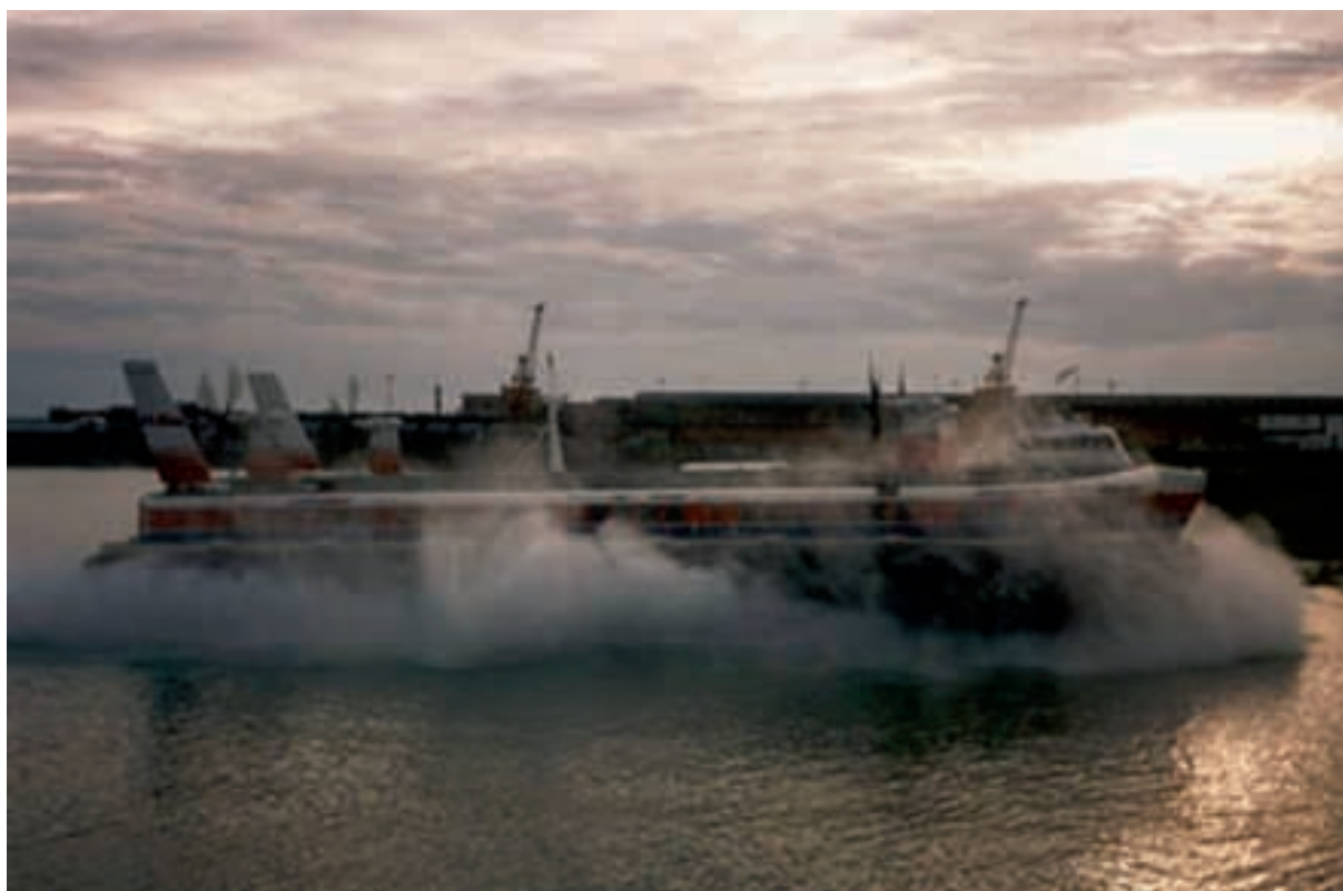
For over 20 years the "stretched" version of the massive, SRN4 hovercraft carried up to 424 passengers and 54 cars between Dover and Calais. (Photo Credit: Rob Fuller)
