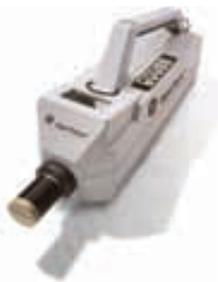
tor. The optional vacuum wand draws vapors into a sponge-like sampler trap, which is then inserted into the unit. The device's on-board computer handles all data logging automatically.
