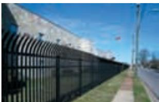
beam posts. The design of the Impasse is intended to provide an effective first line of defense. Special 'break-away' security nuts prevent tampering or removal by conventional tools, and the configuration of the Impasse allows for additional security features such as sensor and alarm systems.
