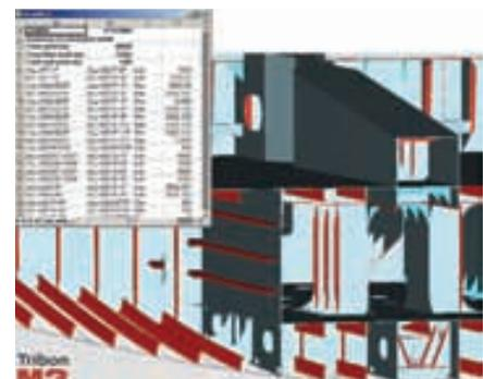
Welds automatically detected and report showing weld lengths and types.
