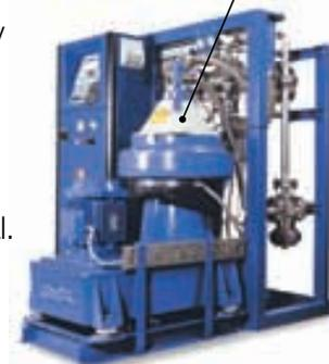
EcoStream is a high-speed centrifugal separation system for bilge water treatment. Without chemicals or absorption filters, it generally reduces oil content to less than 5 ppm – even when emulsions are present.
