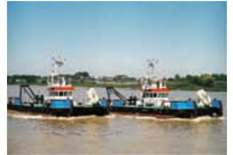
sels will be deployed in the Caspian Sea on a long term contract, supporting the local oil- and gas industry. Because of the local conditions the draft is limited to one meter and despite this limited draft, the vessels have a bollard pull in excess of 9 tons.
