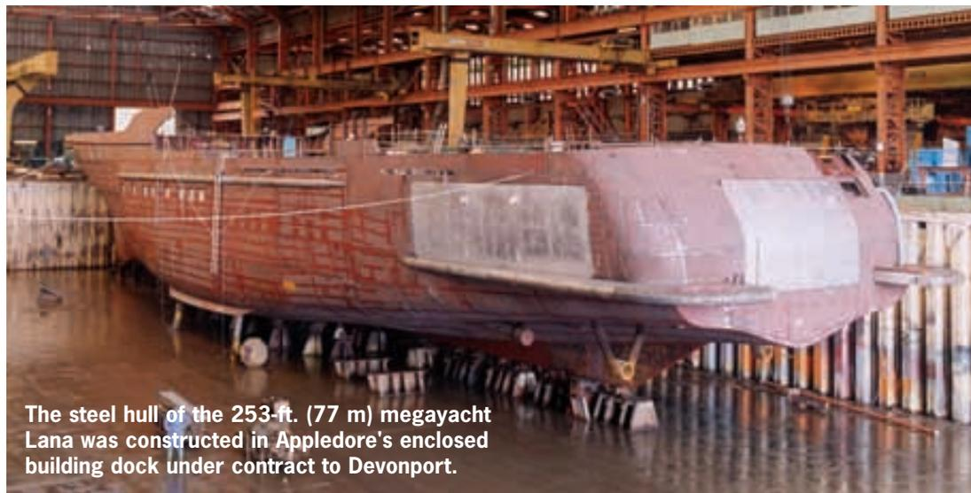
The steel hull of the 253-ft. (77 m) megayacht Lana was constructed in Appledore's enclosed building dock under contract to Devonport.
