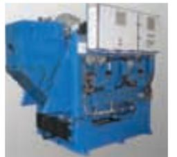
new design sludge burner, making it possible to burn up to two million Kcal/hr. (2,326 kW). The sludge from heavy fuel oil is burned by an atomizing process, which in combination with a high efficiency turbolator mixes the combustion air with the atomized particles even at high capacity.
