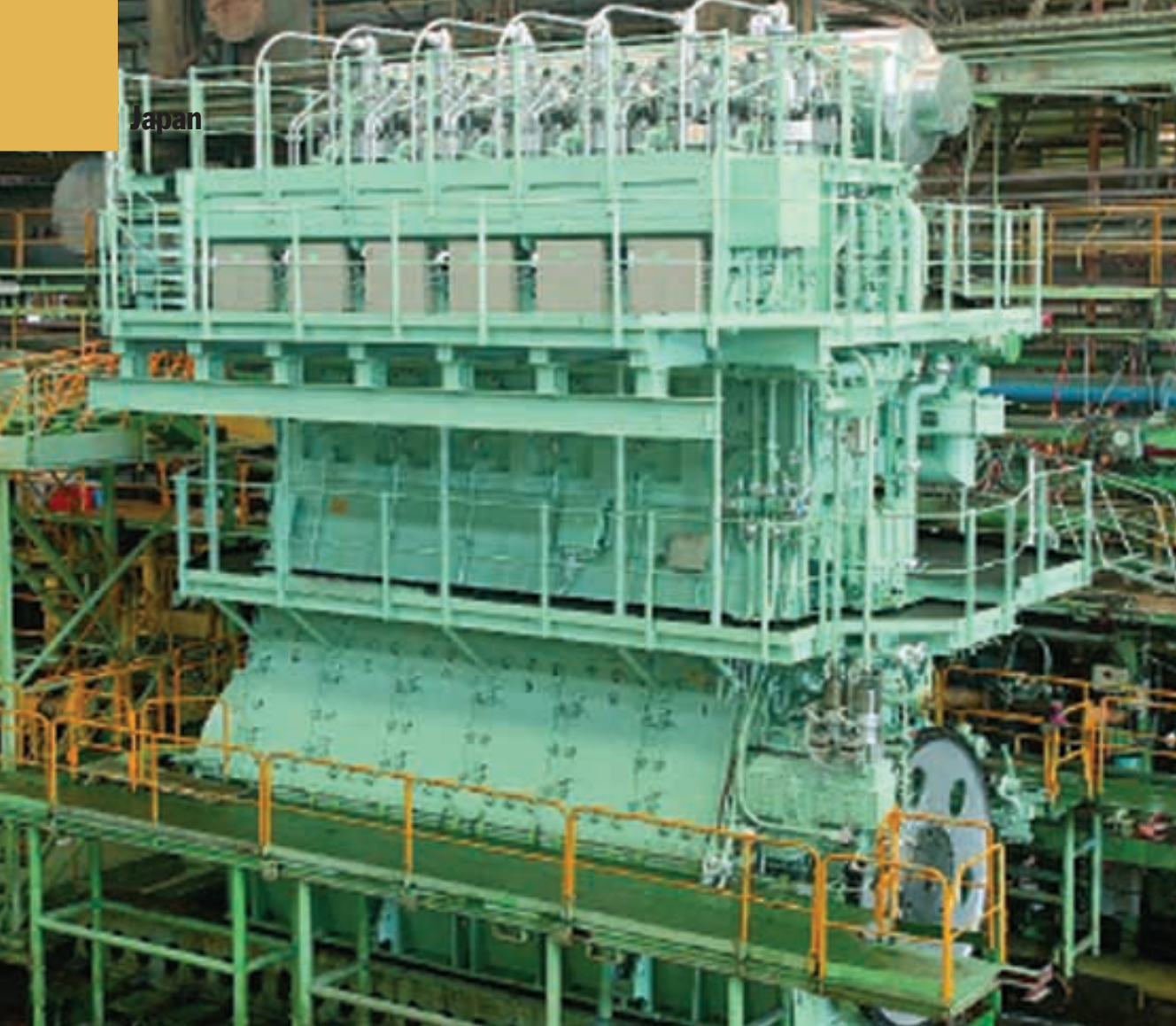
A six-cylinder Sulzer RT-flex 50 marine diesel engine built at Wärtsilä's licensee Diesel United Ltd. in Japan.
