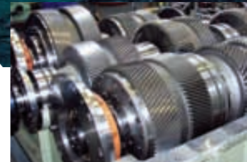
RENK marine gears of the WARP propulsion system for corvettes of the South African Navy
