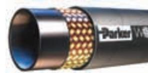
1SN). The 422/421 offers higher working pressures than the existing Parker 421 hose, intended for improved reliability and expanded applications. Additional features of Parker's 422/421 hose include a nitrile inner tube for greater fluid compatibility across a wide range of hydraulic fluids, including biodegradable ones. The hose is available in sizes -4 to -32.
