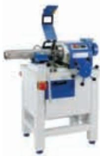
to 17 mm. The standard PBM 4 is fully manual operated. With the heavy duty self-centering prism clamp the pipe is held firmly in place. After starting the motor the tool head can be moved by hand towards the pipe to make a bevel. According to Wortelboer, all these handlings take place in a few seconds. The PBM 4 and other PBM pipe end preparation machines up to diameter 24-in. pipe (O.D. 610 mm).
