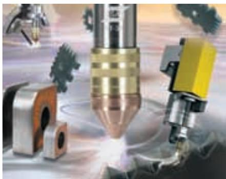
ESAB's m3 Plasma System combines multiple plasma cutting and marking features in a single system. The m3 system aims to deliver high-speed, low-cost standard plasma cutting; high-quality precision cutting and marking; and high-current, thick-plate cutting all with a single plasma torch. When configured for 600-amp operation, the system can cut and mark material from 1 mm to 160 mm with uniform quality.
