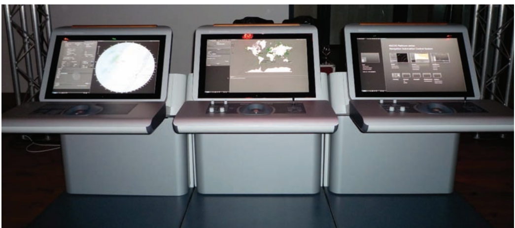
Latest integrated bridge system developments from SAM Electronics include an advanced range of new-generation vessel control systems combining navigation, automation and control functions, NACOS Platinum.
