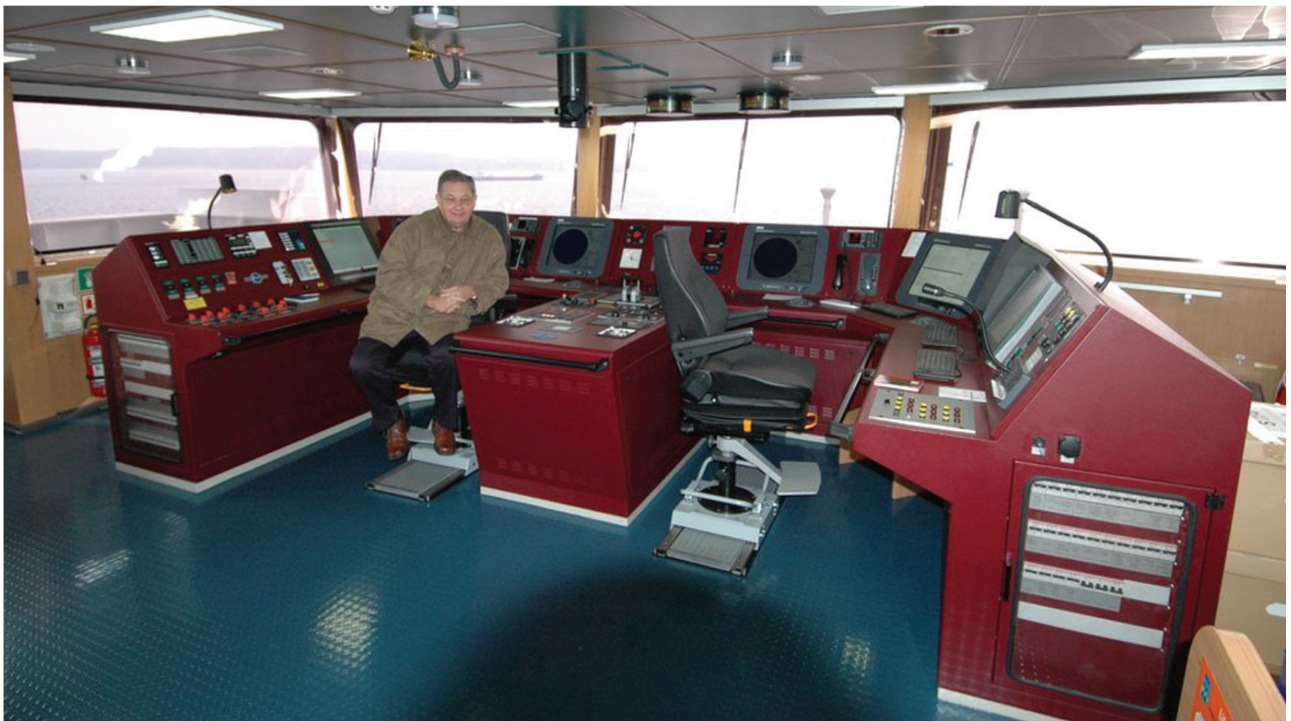
Pictured is the bridge from the "Green Coastal Tanker" MT Seychelles Paradise, which measures 67.8 x 13.2 x 5.2 m and was built by Lindnau for Seychelles Petroleum Ltd. The ship is suitable for the transport of oil and products with flashpoint < 60°C, maximum density 1,025 t/cu. m. and maximum filling temperature 60°C. Six epoxy-coated cargo tanks with smooth surfaces are provided to ensure short discharge times and minimum slop residues.
