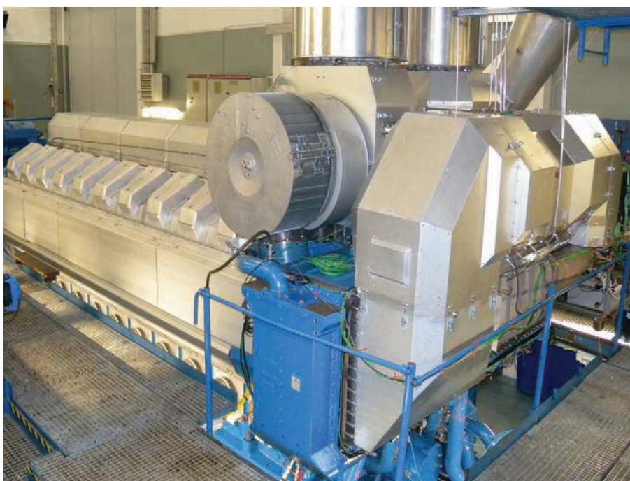
The 2-stage turbocharging technology being tested on a 20-cylinder Wärtsilä 32 engine in the laboratory in Finland.
