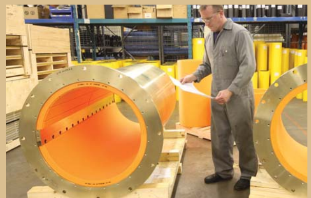
Thordon COMPAC Bearings with tapered key set installed in bronze carriers prior to shipping.
