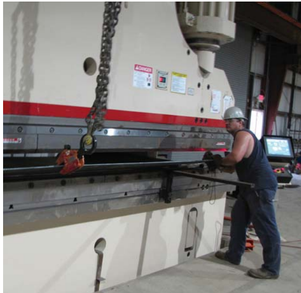
The new $30m McGinnis, Inc. facility in South Point, Ohio features a 1500-ton, 40-ft. tandem press brake from Cincinnati Inc. to help speed barges and towboats back into service. Below are a "Before" and "After" photo of a recent job.
