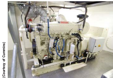
Left The QSK19 powered gen set to supply the cargo pump and bow thruster.
